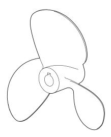
In all cases, the propeller should allow the engine to reach its rated rpm with the maximum boat load.
