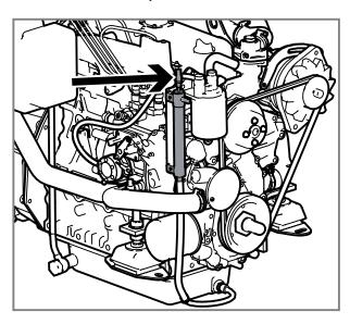
**4.** Suck out all the oil using the oil drain pump. Remove the drain hose and lock the pump.
